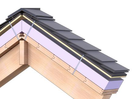
Our current roof gets too hot! This places a burden on our cooling systems and prematurely ages the roofing materials. As illustrated here, space will be created for airflow, resulting in longer life for the shingles. Our renovation will allow us to install commercial grade materials that have a longer replacement life.
